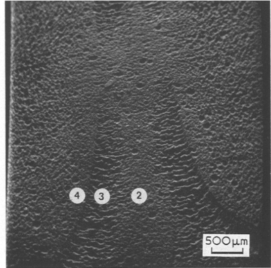
Figure 5 Polyethylene weld after etching for 12 h in chromic acid at 67°C. Magnification \times 17 . (Scale bar = 500 \mu\text{m} .)
